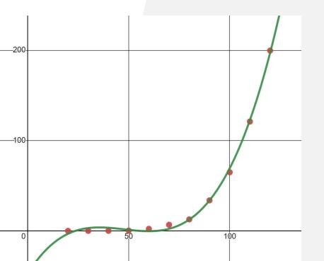
By running the algorithm 10 times each across N =  $\{20, 30, 40, 50, 60, 70, 80, 90, 100, 110, 120\}$  and averaging, we can create a plot of N vs. time (left). A regression analysis of various sizes of N shows that a cubic polynomial fits the data with a 0.998 R Squared value. This highly indicates that this algorithm runs at O(N^3) time.
