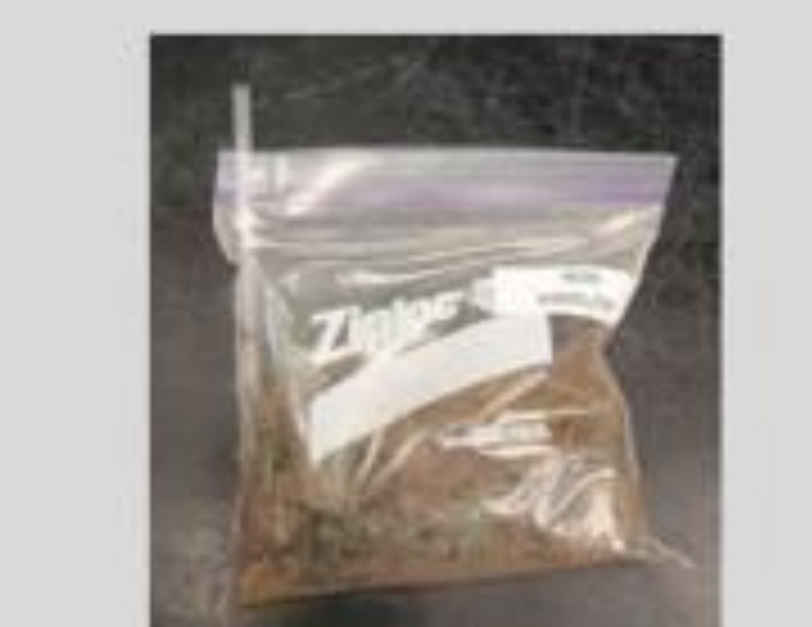
Figure 4. Plastic bag containing soil, water, and plant tissue for incubation. A plastic straw was inserted into the bag to insure optimum air flow into the bag.
