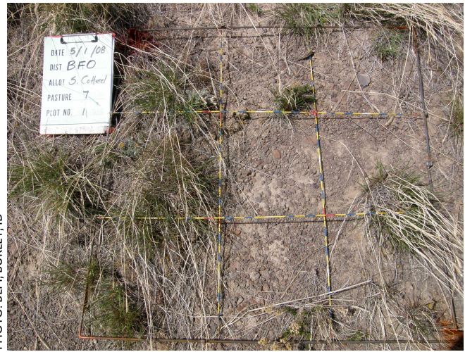
Figure 5. A permanent grid frame such as those used by federal land-management agencies. Each square is 1 foot x 1 foot. Diagonal corners are painted different colors so the photographer knows where to stand.
