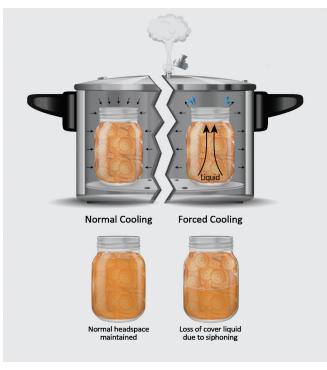
**Figure 20.** This diagram illustrates the importance of allowing the canner to cool normally, without force cooling. The jar on the left has equalized pressure inside and outside. When the canner cools gradually, the pressure remains equal. Note how the jar on the right is losing liquid due to the rapid depressurization of the canner. Higher pressure inside the jar forces liquid out.
