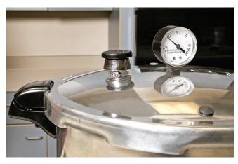
Figure 19. Allow the canner to depressurize normally without assistance.
