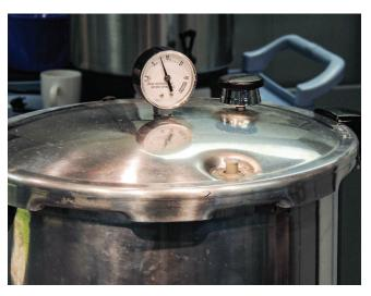
**Figure 6.** The dial gauge is a delicate instrument and must be tested each year for accuracy. Courtesy of Colorado State University.
