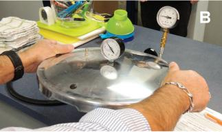
**Figure 7.** A, dial-gauge testing unit. B, comparison of canner gauge to master gauge.
