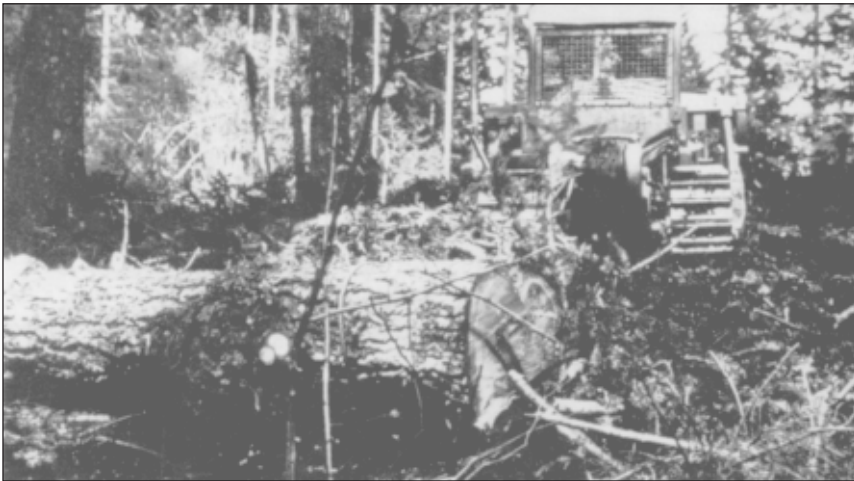
Figure 6.—To reduce the area of compacted soil, the logger pulls line to the log (above) and then winches it to the vehicle on the designated skid trail (below).
