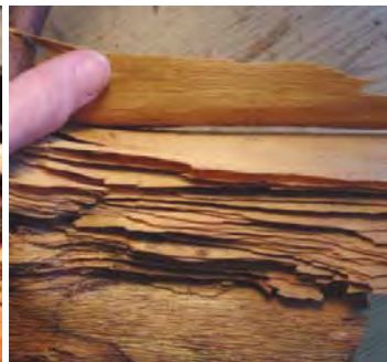
Fig 4. Examined longitudinally, wood decayed by Phellinus weirii separates easily into thin concentric sheets.
