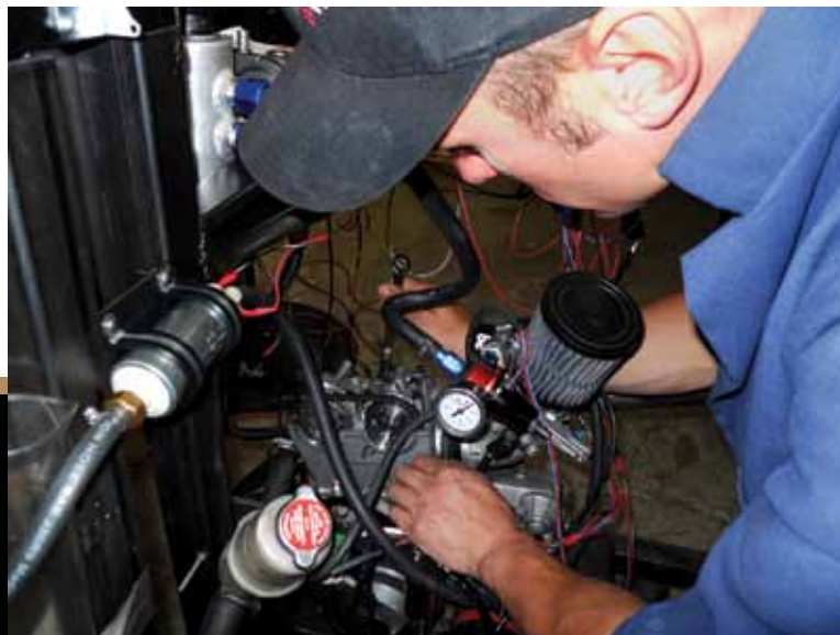
Zack Porter is preparing to reattach the valve cover to the top of the engine. This cover holds one of the two sensors necessary to run the engine with a fuel-injected system.
