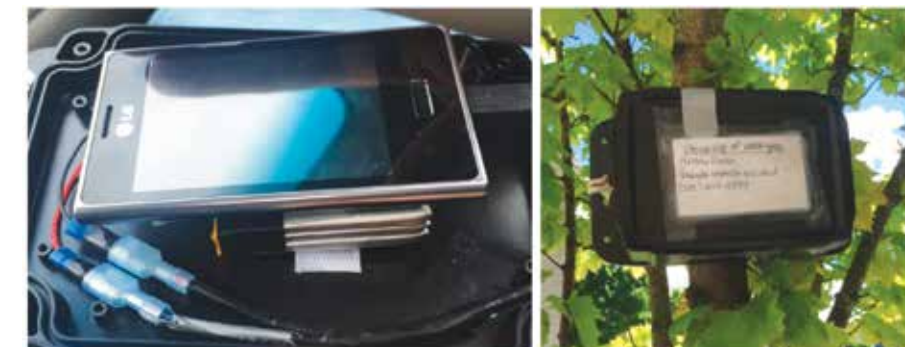
(a) Sensor with auxiliary battery (b) Sensor placement. Static sensor setup and placement
