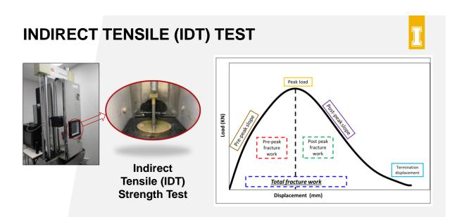
I A compressive load at a constant rate of 50±5 mm per minute until failure
