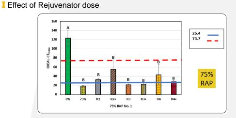
Some rejuvenators like R2, had a favorable effect on the cracking resistance as the dose increase while other like R4 adversely impacted the cracking resistance
