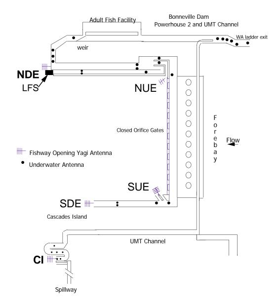
Figure 3. Dam diagram of underwater and aerial antennas used at Bonneville Dam to monitor movements of radio-tagged Chinook and sockeye salmon in 2013 and 2014. Solid square indicates the location of the modified north downstream entrance (NDE) and lamprey flume system (LFS). Note that the Bradford Island fishway is not shown.
