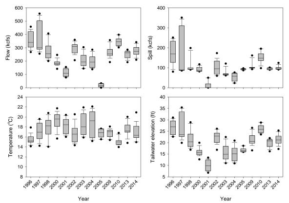
Figure 40. Box plots of the total discharge ('flow'), spill, water temperature, and tailwater elevation on the days that radio-tagged adult summer Chinook salmon first approached the Cascades Island fishway opening. Distributions show 5<sup>th</sup>, 10<sup>th</sup>, 25<sup>th</sup>, 50<sup>th</sup>, 75<sup>th</sup>, 90<sup>th</sup>, and 95<sup>th</sup> percentiles.
