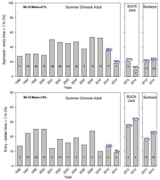
Figure 23. Percentages of radio-tagged summer Chinook and sockeye salmon that took > 1 h to pass from the north downstream approach to fishway entrance and from opening to the base of the ladder. Sample sizes are inside each bar.
