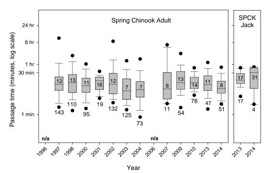
Figure 41. Spring Chinook salmon passage time distributions (plotted on log-scale) from Cascades Island fishway entry to the antenna at the base of the ladder (not monitored in 1996 and 2006). Numbers inside boxes are median times. Distributions show 5<sup>th</sup>, 10<sup>th</sup>, 25<sup>th</sup>, 50<sup>th</sup>, 75<sup>th</sup>, 90<sup>th</sup>, and 95<sup>th</sup> percentiles; sample sizes are below boxes.
