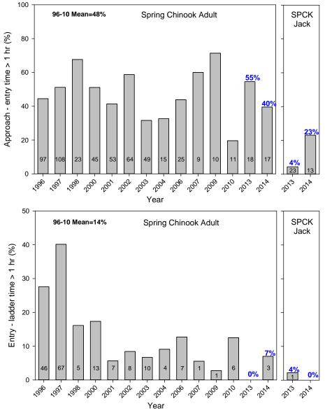
Figure 22. Percentages of radio-tagged spring Chinook salmon that took > 1 h to enter the north downstream fishway entrance (top panel) and the time to pass from the fishway opening to the base of the ladder (bottom panel). Sample sizes are inside each bar.
