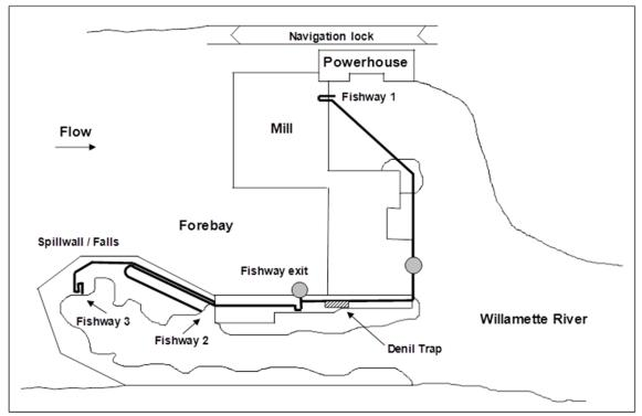
Figure 2. Schematic drawing of Willamette Falls Dam, Oregon, showing the location of three fishways, the two fixed-location radio receiver sites (•) deployed at the dam in 2012. Additional antennas were located in the dam tailrace (0.5 km downstream).
