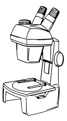
In some cases, it is better to work with less magnification. This is true when the objects are opaque and too large to be seen whole under the lowest power of the compound microscope. Because the working distance is much greater, it is also possible to handle objects while they are being viewed with this microscope. Specimens are usually viewed by reflected light, and since there are two objectives and two eyepieces, a 3-dimensional effect is achieved.
