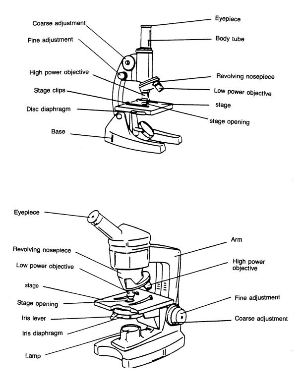
7. Underneath the stage is a diaphragm. The diaphragm regulates the amount of light entering the microscope. The diaphragm is adjustable for the type of lighting conditions used.
