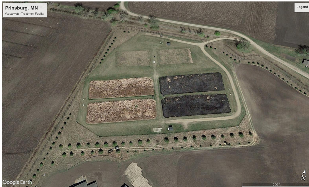
Figure 14. Aerial image of Prinsburg, Minnesota's wastewater treatment wetlands for a population of 497 (Google Earth, 2018).
