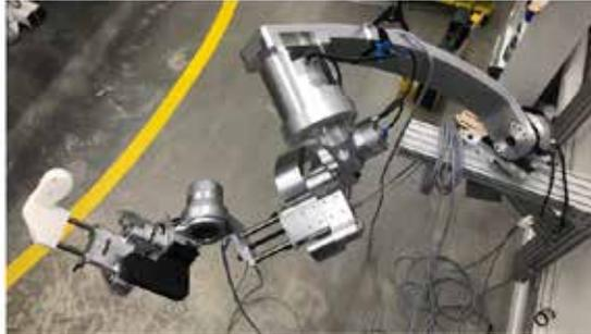
calculation, and motor commands are performed at a sufficiently high rate (~1000 Hz), the exoskeleton can effectively be used as an assessment instrument to measure user mobility, or provide assistive support forces.
