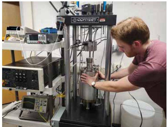
Graduate student Colin Burkhalter demonstrates the apparatus designed to performed fatigue and corrosion tests at high temperature and pressure using a high purification water circulation loop.
