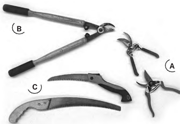
Figure 4. Tools used to prune woody plants include (a) bypass hand shears, (b) bypass loppers, and (c) handsaws. Photo by Robert Tripepi.
