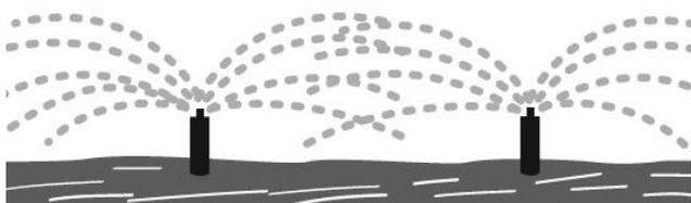
**Figure 5.** Sprinkler overlap to provide head-to-head coverage.
