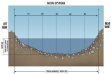
Figure 31. Accurate measurements along your stream transect will allow you to track changes in channel migration and the effects of sedimentation in your stream. *Courtesy of Noah Kroese.*
