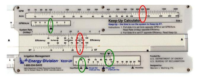
Figure 5. Keep-Up calculation for center pivot and linear move systems.
