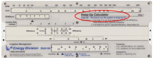
Figure 2. Keep-up side of slide rule.
