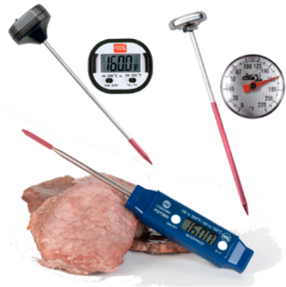
Figure 1. A dial instant-read thermometer (right) displays the temperature sensed in the bottom 2 inches of its stem. Digital instant-read thermometers (left and bottom) display the temperature sensed in the bottom ½ inch of its stem. A thin-tipped thermometer (bottom) senses the temperature in thin meat.
