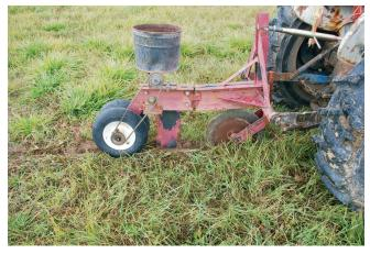
Figure 23. Burrow-builder applicator. Photo by Glenn Shewmaker.
