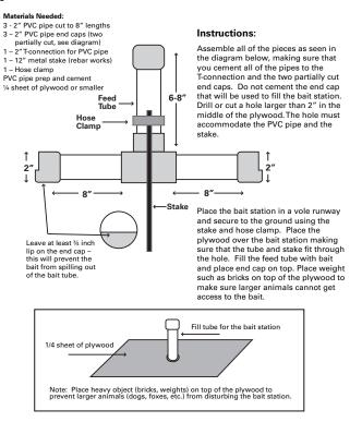
Figure 7. Bait station construction. Diagrams by Sherman Takatori.
