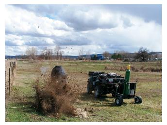
Figure 25. Use of the Rodenator to control pocket gophers. Photo reproduced courtesy of Meyer Industries, Emmett, Idaho.
