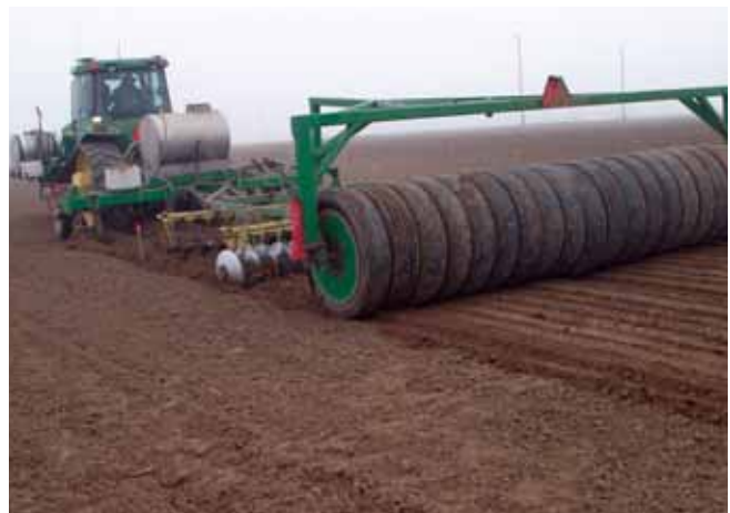
Figure 3. Telone II applicator, disc and soil compacter
