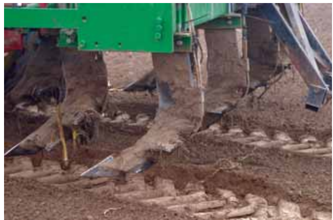
Figure 2. Ripper shank for Telone II application
