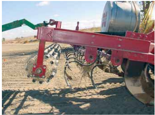
Figure 1. Ripper type soil fumigator for Telone II application
