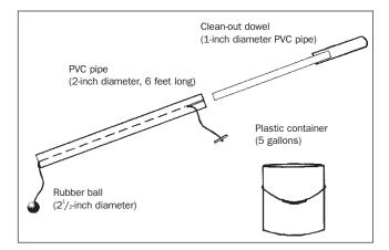
**Figure 2.** Composite sampler for slurries and lagoon sludge or settled solids includes a collecting PVC pipe and a clean-out dowel (smaller PVC pipe), string, and a rubber ball big enough to cover one end of the collecting pipe.
