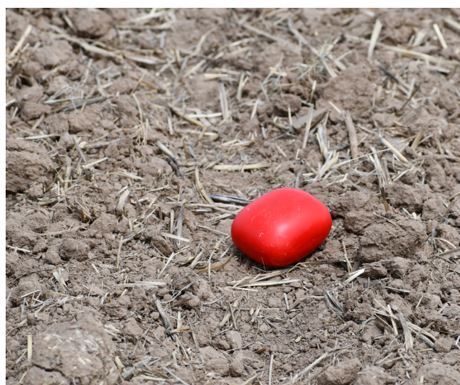
Figure 4. Example of an instrumented sphere [Techmark Impact Recording device (IRD)] placed on top of the soil to be harvested with potatoes to monitor the impacts during harvest.
