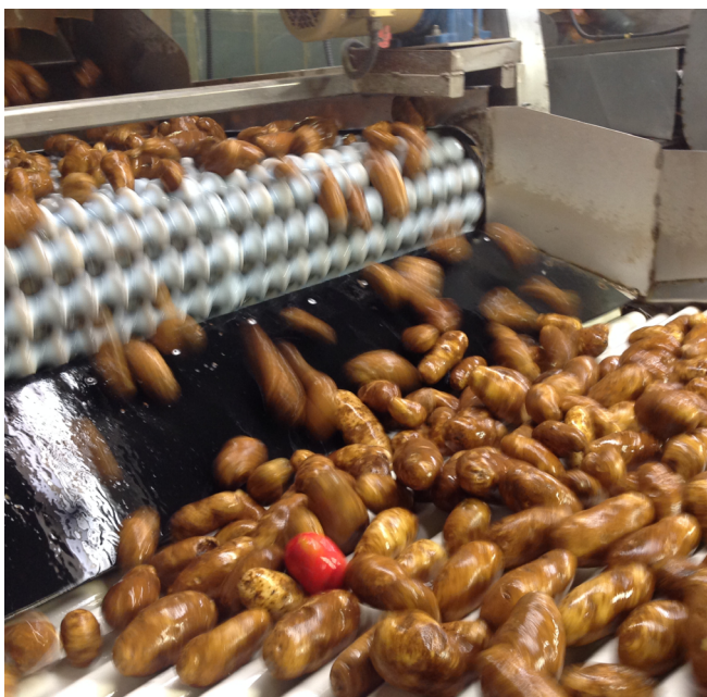
Figure 5. An IRD (red ball) recording impacts as potatoes are being conveyed in a fresh pack operation.
