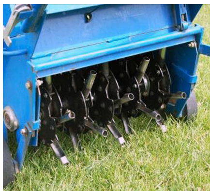
Figure 2. A hollow-tine core aerator (note the hollow tubes sticking out of the coring mechanism) is the preferred piece of equipment to most effectively aerate a lawn.
