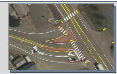
Significant improvements are possible at the Highway 55/Lake Cascade Parkway intersection. The west leg of the intersection is over 120 feet wide, has high speed turning radii, and sees many large vehicle types including motorhomes and truck/boat set ups. Narrowing the crossing, elevating the pedestrian profile, and defining the travel spaces may improve the overall safety of the intersection and promote walking trips as sought by the residents of and visitors to Cascade.
