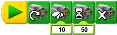
The program will set the time frame for our observations. This way we don't need a separate clock. Make adjustments to the motor power (“10” in the image above) for each trial. Count the number of full turns the propeller makes at each power setting and record in the table below.
