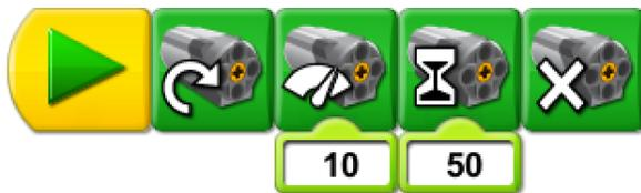
The program will set the time frame for our observations. This way we don't need a separate clock. Make adjustments to the motor power (“10” in the image above) for each trial.
