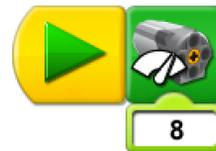
Is it hard to see a difference in the settings? Try different speeds and describe the differences. Youth will be able to notice that the motor turns faster, but a limitation is being able to be more accurate about the movement. For instance, how much faster is the motor at setting 5 vs. 3, or 9 vs. 2? We will also notice that it is hard to see (observe) the rotations because the part turning is so small and uniform.
