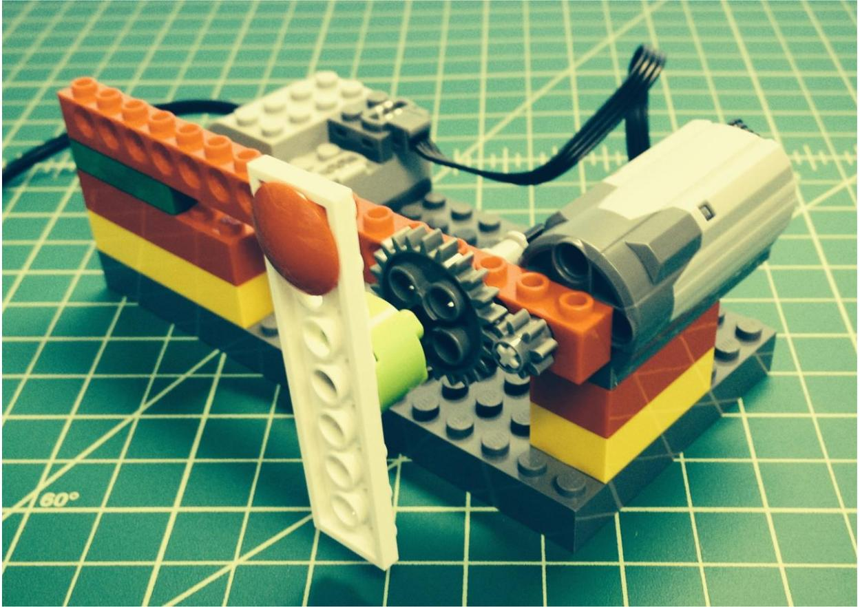
**Test #2.** Number of turns when small gear drives large gear
