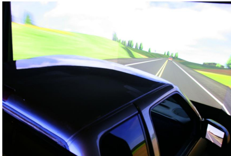
Figure 1 Overhead view of the Driver Simulator Chevy S-10 cab with the 3 Main forward displays and right-side mirror display
