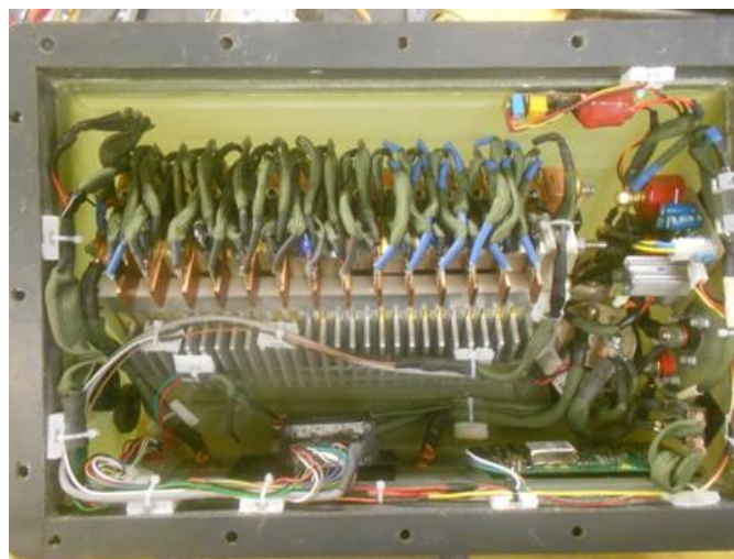
Figure 6: Fully assembled battery pack.
