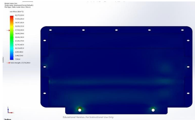
Figure 7: Finite element analysis showing the bottom of the battery box.
