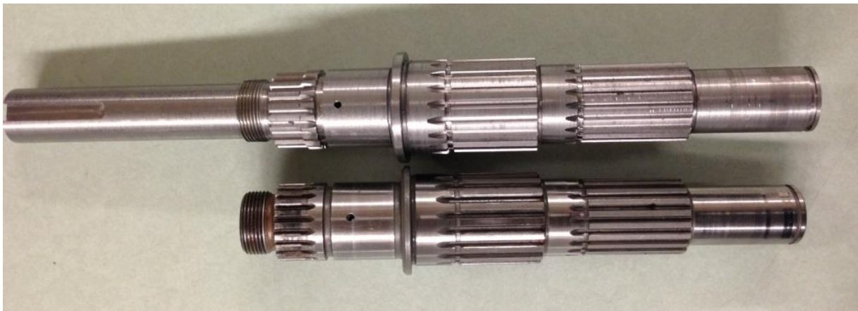
Figure 16: Custom (top) and stock (bottom) output shafts.
