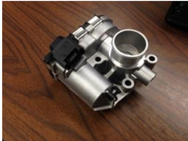
Figure 8: Bosch 32mm throttle body.
