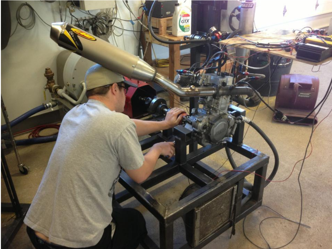
Figure 24: Dynamometer testing setup.
