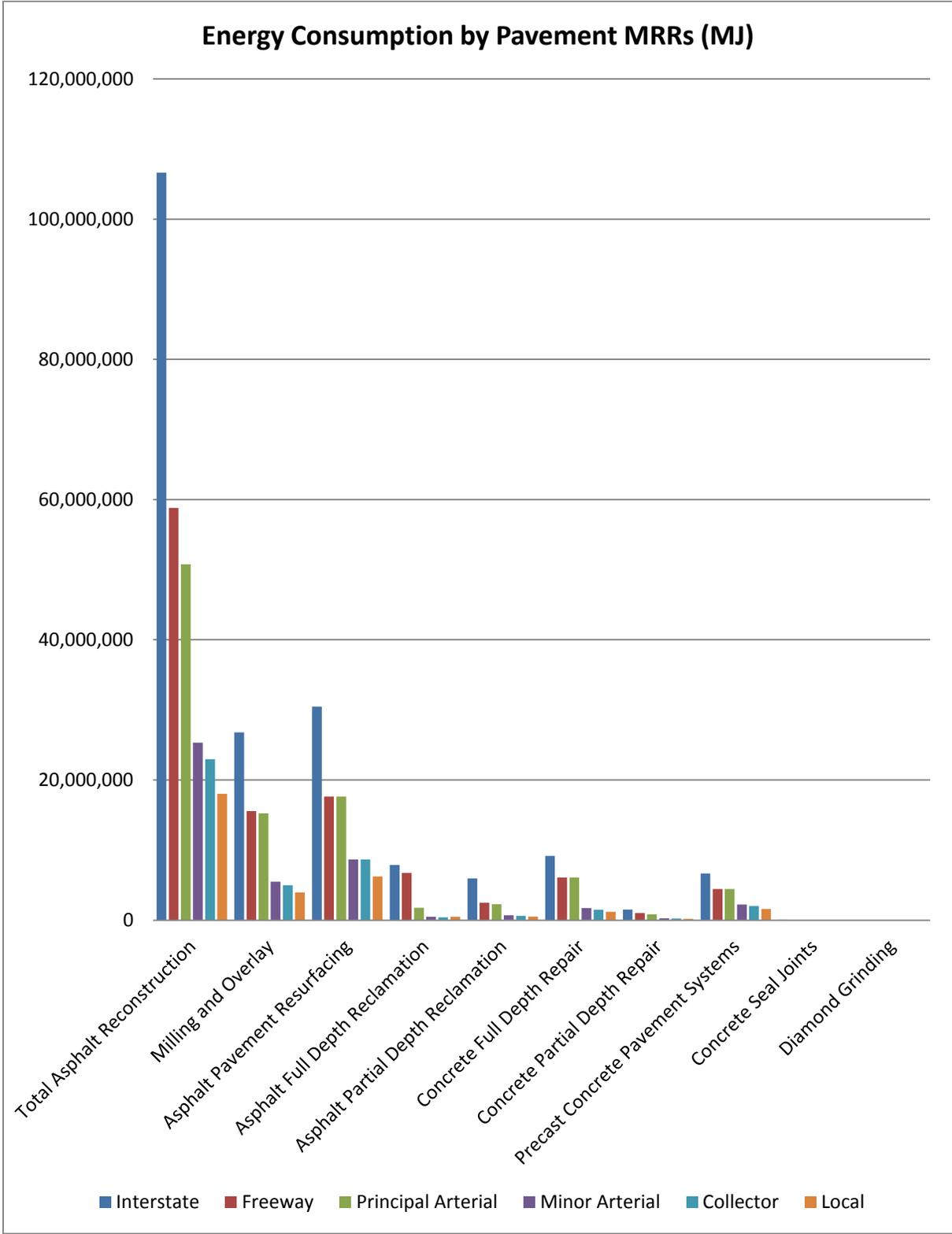
Figure 22: Energy Consumption of Pavement MRRS over the Design Life of Pavement (for one lane km)
