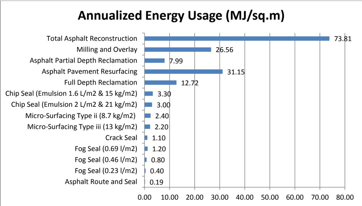
Figure 18: Annualized Energy Usage for Flexible Pavement MRR techniques
