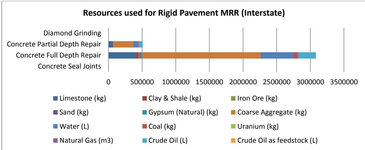
Figure 11: Resources used for Rigid Pavement MRR (Interstate)
