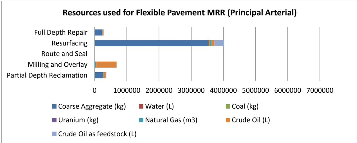
**Figure 7: Resources used for Flexible Pavement MRR (Principal Arterial)**
