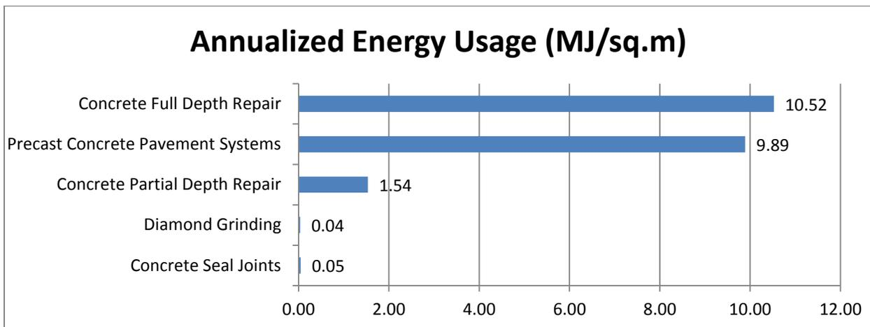
Figure 20: Annualized Energy Usage of Rigid Pavement MRR Techniques
