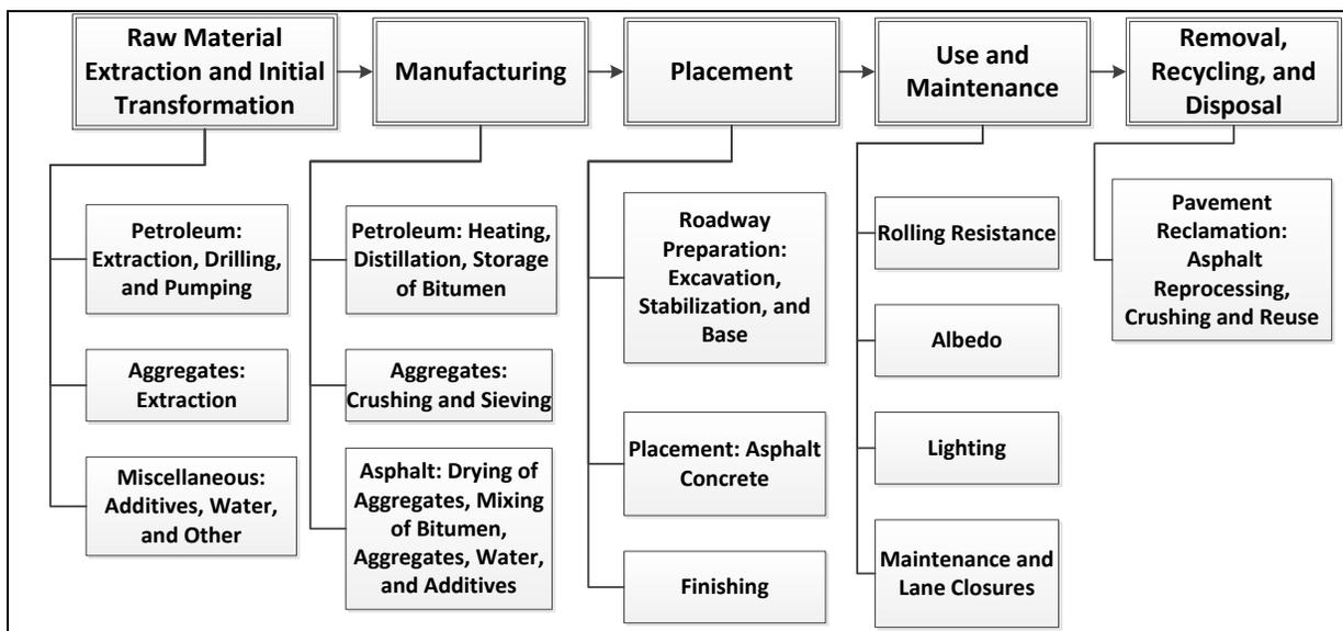
Figure 4: Life Cycle Phases and Components for Flexible Pavements (Loijos, 2011)
