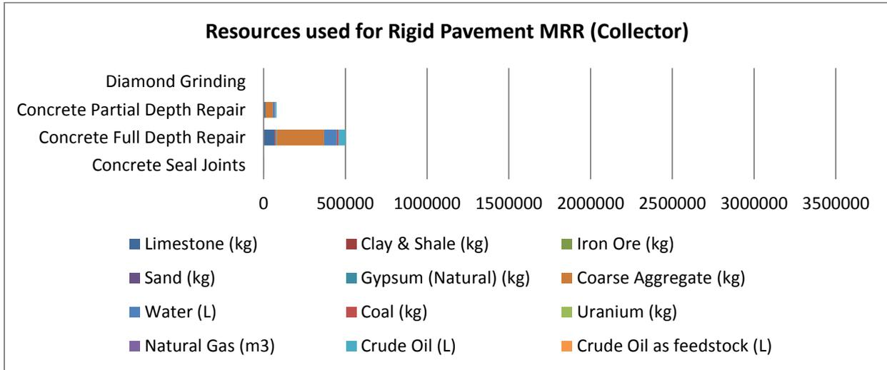
Figure 15: Resources used for Rigid Pavement MRR (Collector)
