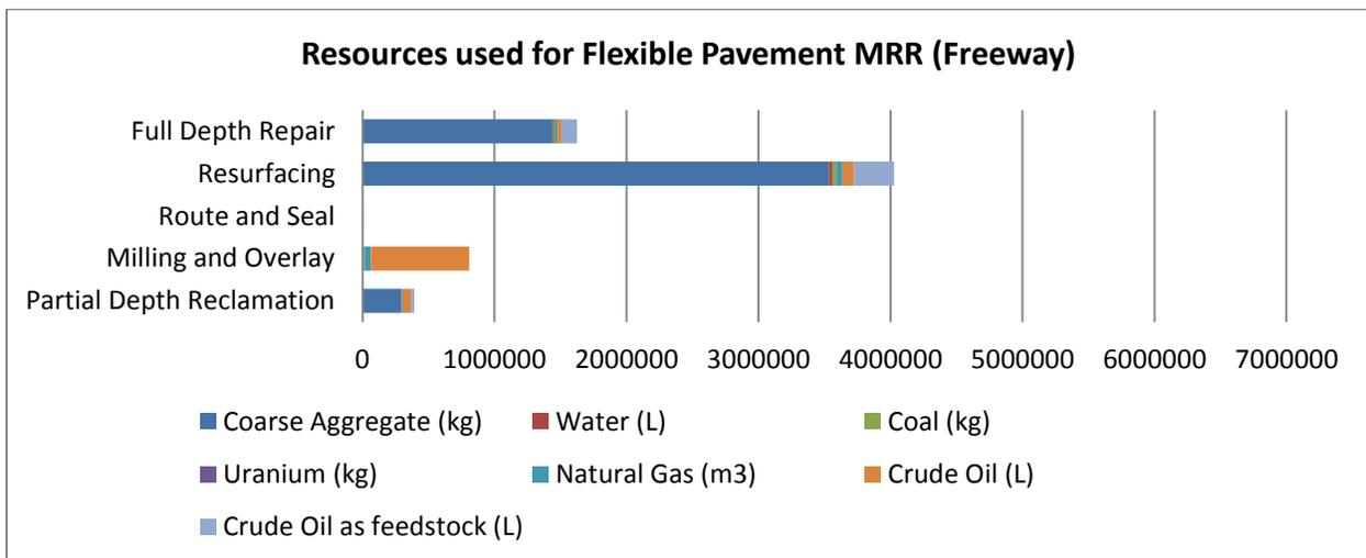
Figure 6: Resources used for Flexible Pavement MRR (Freeway)
