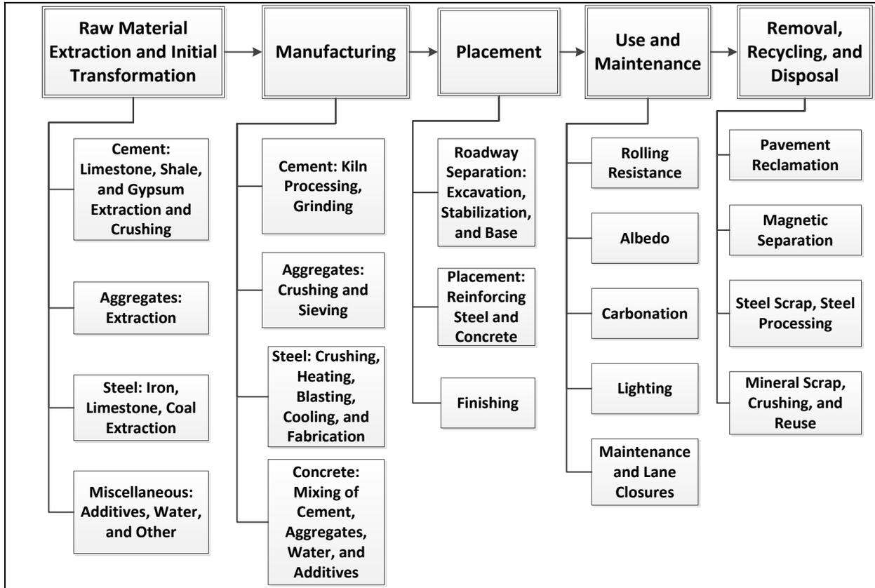
Figure 3: Life Cycle Phases and Components for Rigid Pavements (Loijos, 2011)
