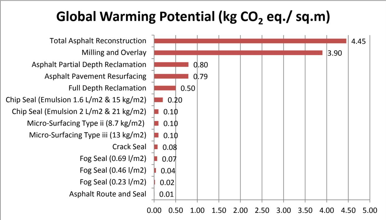
Figure 17: Global Warming Potential for Flexible Pavement MRR techniques
