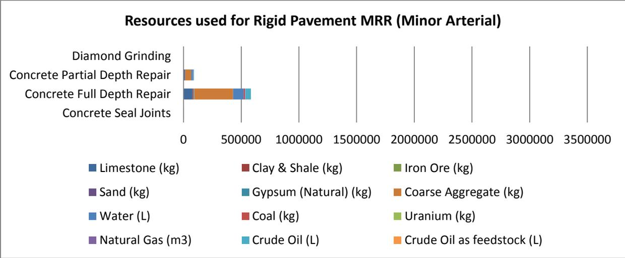
Figure 14: Resources used for Rigid Pavement MRR (Minor Arterial)
