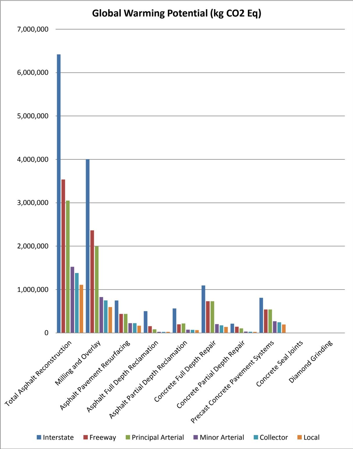
Figure 21: GWP of Pavement MRRS over the Design Life of Pavement (for one lane km)
