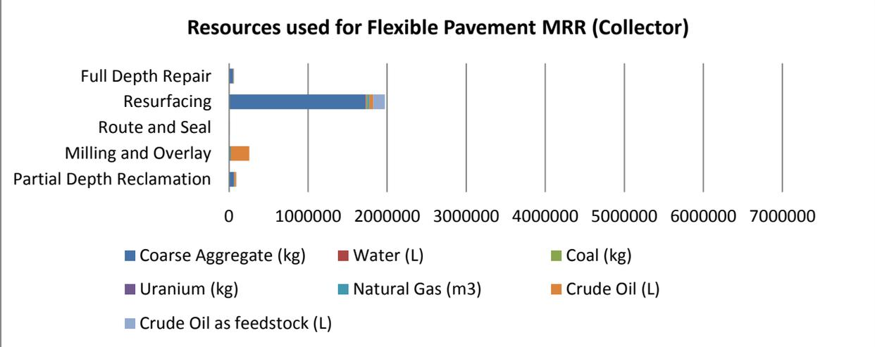
Figure 9: Resources used for Flexible Pavement MRR (Collector)
