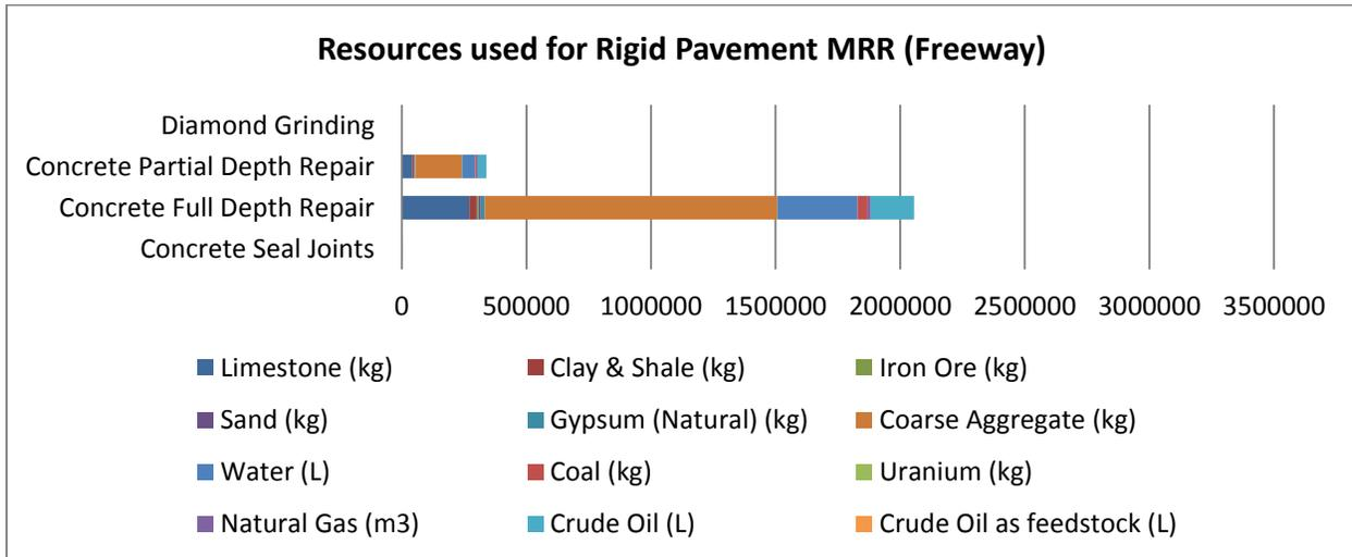
Figure 12: Resources used for Rigid Pavement MRR (Freeway)
