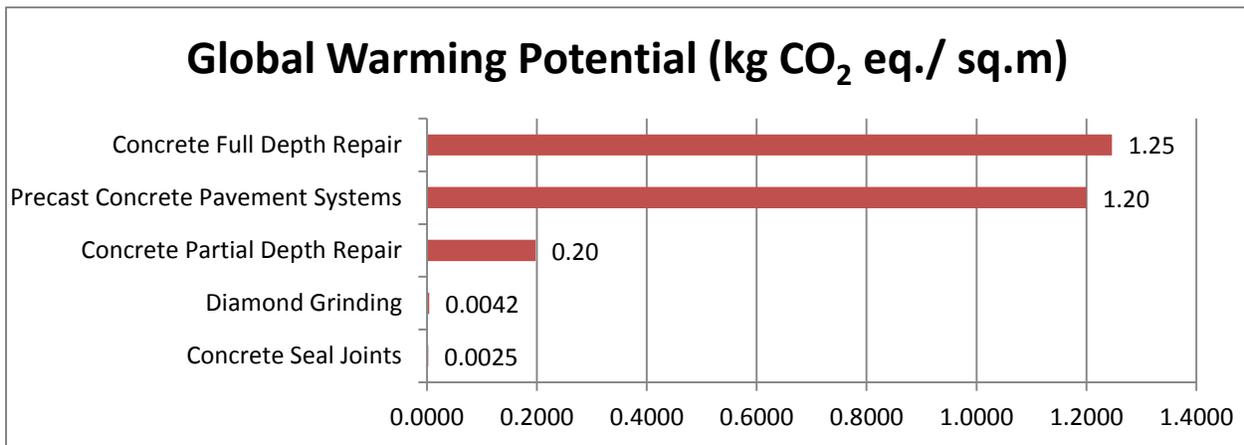
Figure 19: Global warming Potential of Rigid Pavement MRR Techniques
