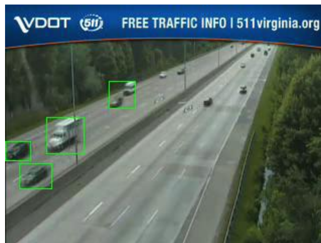
Figure 9. Detected vehicles under heavy compression — realistic video 2, example frame 3
