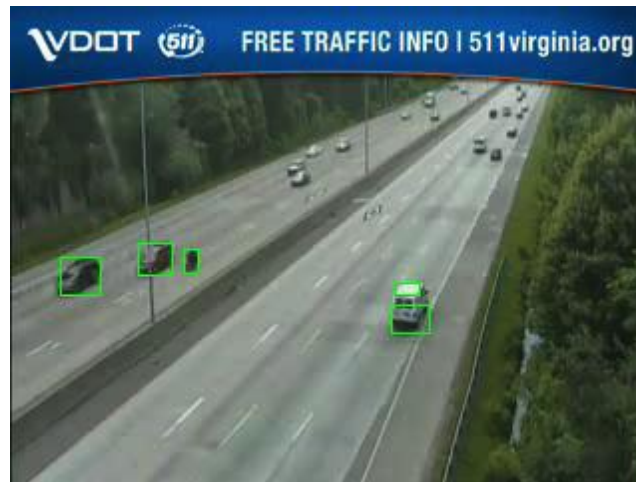
Figure 8. Detected vehicles under heavy compression — realistic video 2, example frame 2
