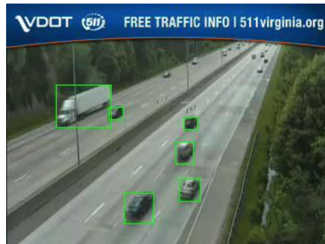
Figure 7. Detected vehicles under heavy compression — realistic video 2, example frame 1
