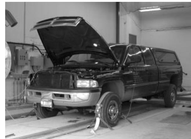
*Biodiesel van undergoing testing on chassis dynamometer.*
