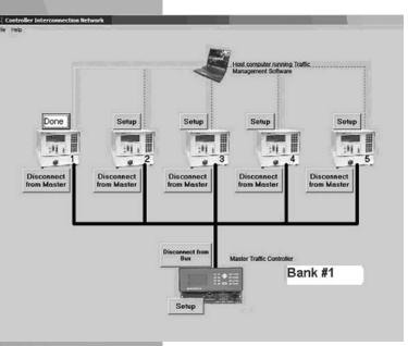
An embedded-controller approach was used for the hardware design because this approach enables easy modification. A GUI displays the status of the network and allows the user to make changes in network configuration.
