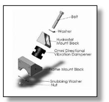
Figure 5 Design of the hydraulic mount system.
