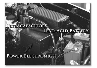
Figure 4 The system installation in a Ford Explorer consists of a bank of six capacitors weighing 0.42 lbs each, a DC/DC converter and controller and a small battery.
