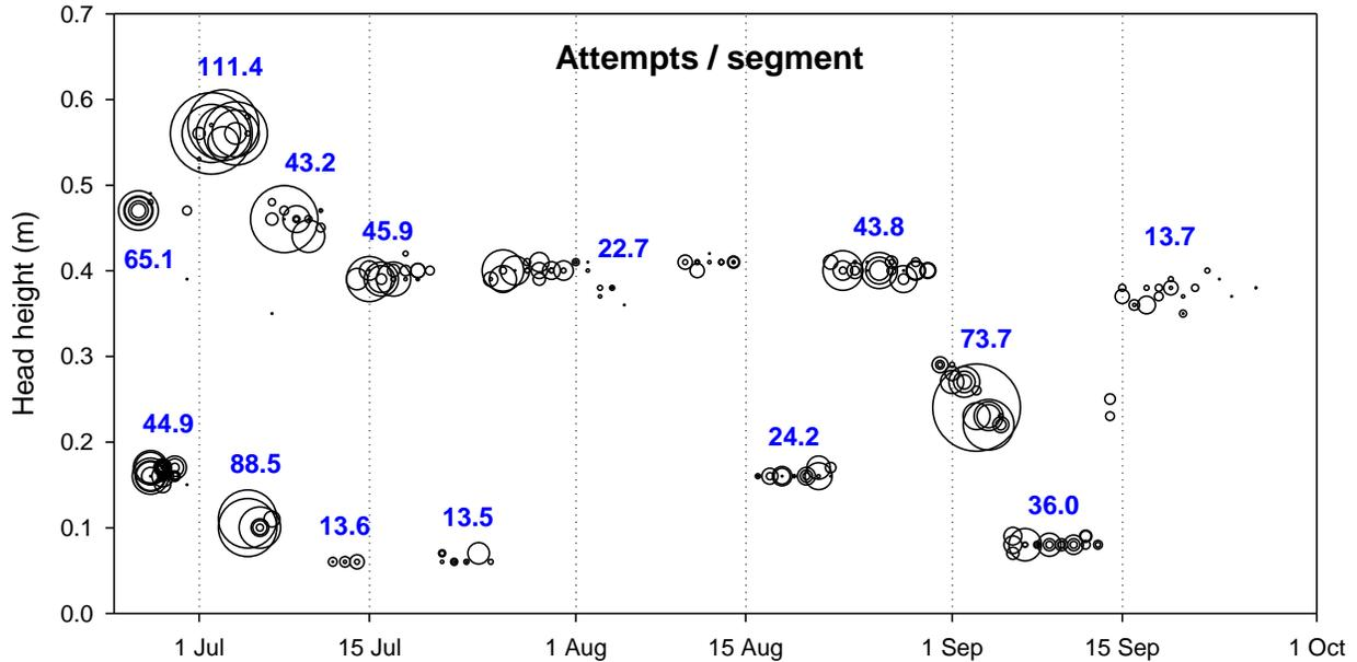
Figure 25. Bubble plot showing the relationships among the number of attempts at the pre-sort pool weir (bubbles scaled to show relative number of events), date, and fishway head (m) in 2017. Blue numbers show the attempts/h for groups of days with similar head treatment.
