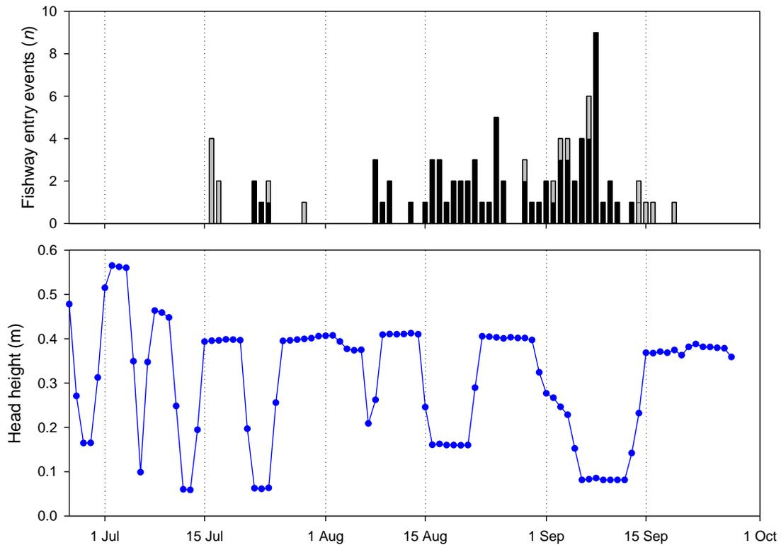
Figure 18. Daily numbers of fishway entry events recorded for radio-tagged adult Chinook salmon at the main fishway opening (black bars, top) and side fishway opening (gray bars, top) and mean daily fishway head height (bottom) in 2017. (See Figure 12 for hourly head height data.)
