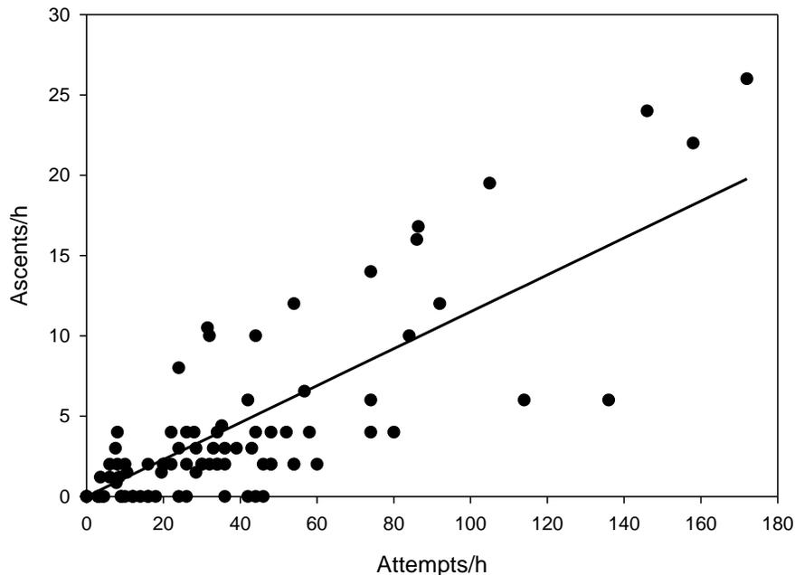
Figure 22. Relationship between the daily attempt and ascent rates (hourly) calculated for adult salmonids at the pre-sort pool weir in 2017. Line is linear regression, forced through the origin.
