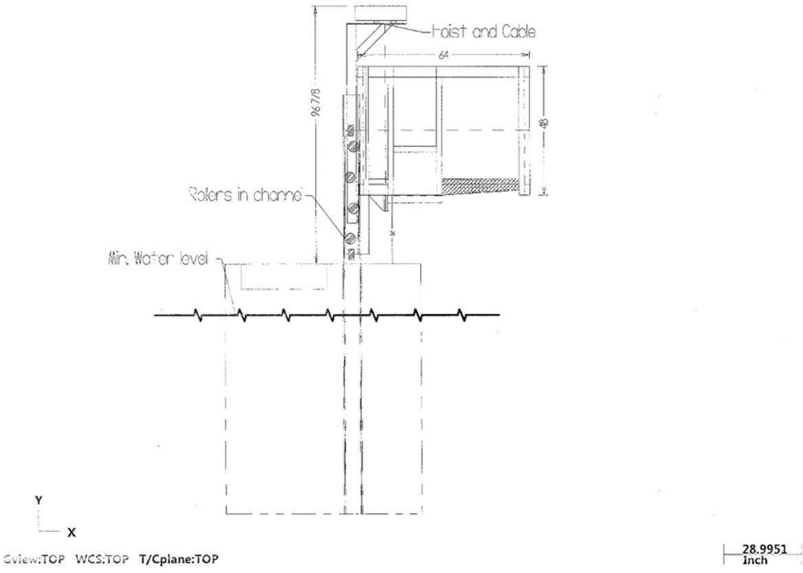
Figure A11. Rollers in channel and hoist and cable.
