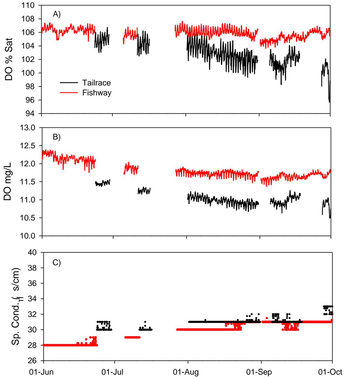
Figure 10. Water chemistry parameters collected in the Foster AFF fishway and tailrace: A) dissolved oxygen percent saturation (DO % Sat), B) dissolved oxygen (DO), and C) specific conductivity (Sp. Cond.) in 2017.
