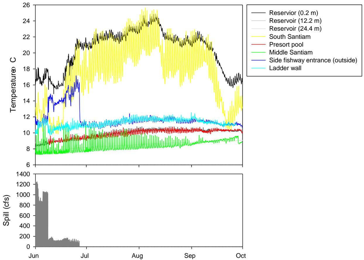
Figure 6. Foster Reservoir, South Santiam (Menear's Bend), Middle Santiam (Sunnyside), and Foster Dam mean hourly water temperatures (top panel) and spill (bottom panel) between 1 June and 1 October 2017. Spill and juvenile fish weir operations were stopped on 26 June.
