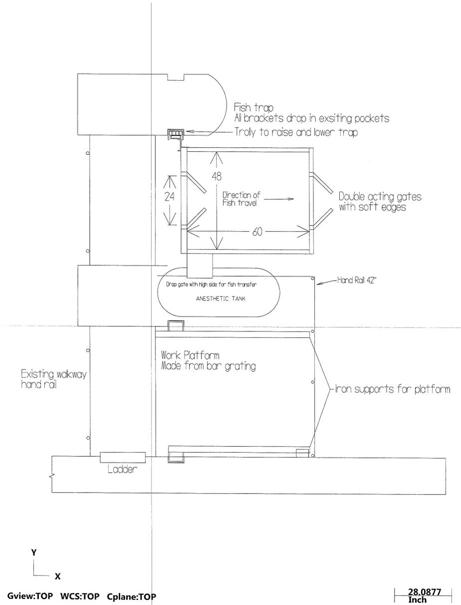
Figure 13. Plan view schematic of the new Lebanon Dam adult fish trap. Measurements in inches.
