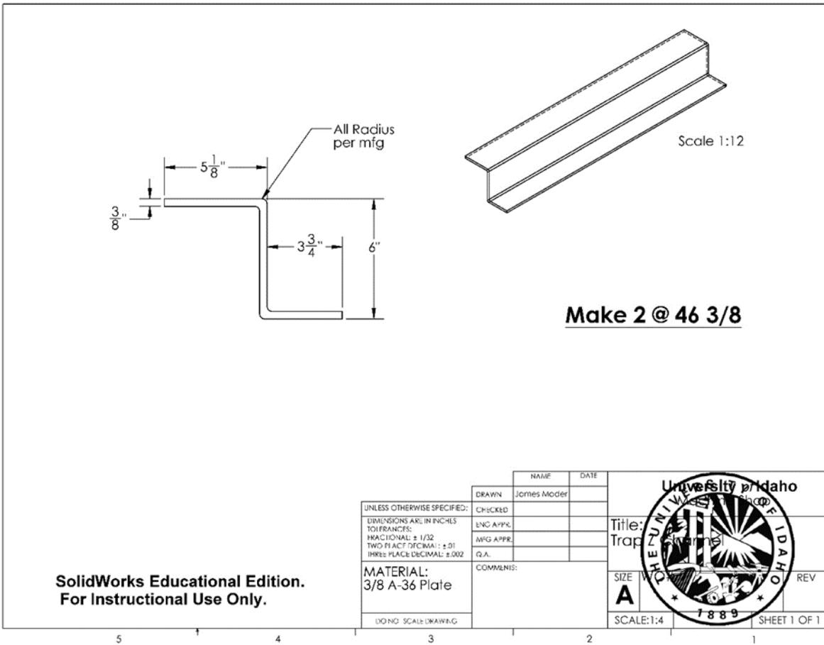
Figure A16. Trap Z channel.
