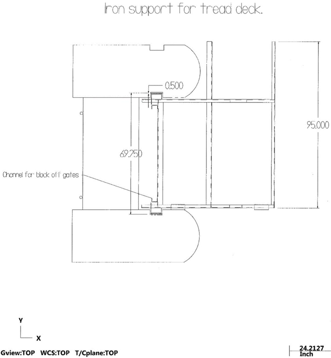
Figure A1. Iron support for tread decking.
