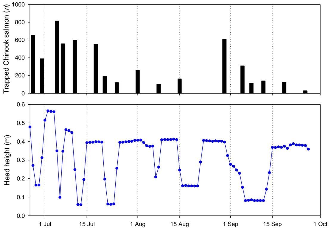
Figure 20. Daily numbers of adult Chinook salmon processed at the Foster Trap (top) and mean daily fishway head height (bottom) during the optical video evaluation in 2017 (26 June to 1 October). See Figure 12 for hourly head height data.
