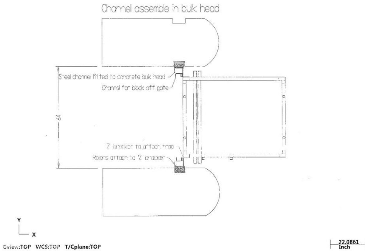
Figure A10. Channel assembly in fishway bulkhead.
