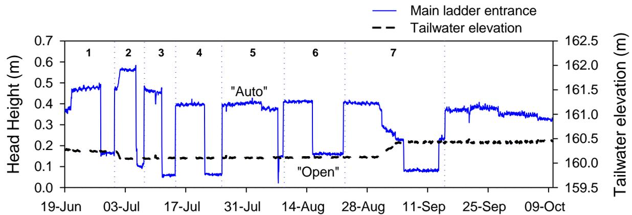
Figure 12. Head height (hourly) at the main entrance ladder in 2017 indicating ‘Auto’ when the weir gate was partially raised (head ~0.46 m [ $\sim$ 1.5 ft]) and ‘Open’ treatments (head ~0.15 m [ $\sim$ 0.5 ft]) when the weir gate was lowered completely during the treatment period (19 June until 25 September). Dotted vertical lines and numbers represent the 7 treatment blocks during the study period. Tailwater elevation referenced to NGVD 29.
