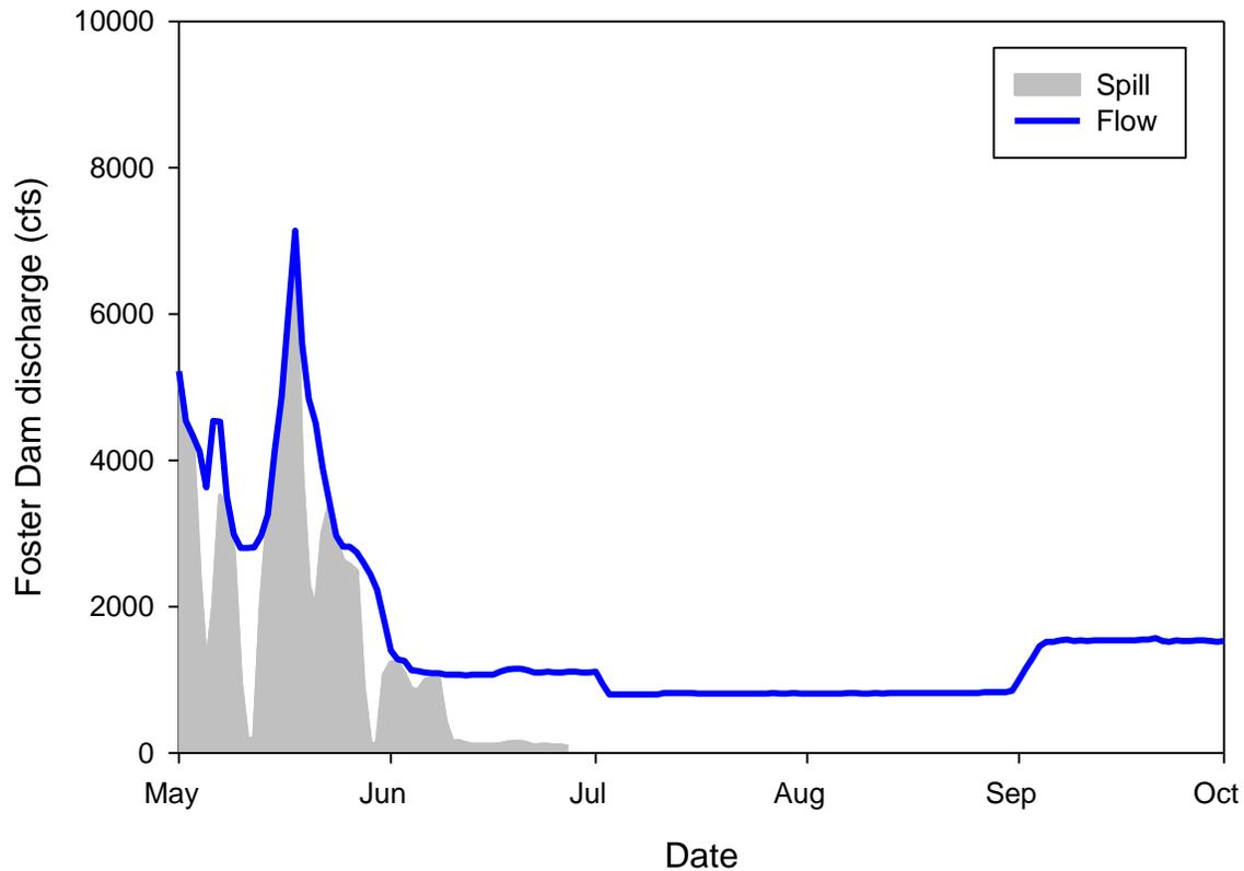
Figure 11. Mean daily flow and spill (cfs) at the Foster AFF in 2017.
