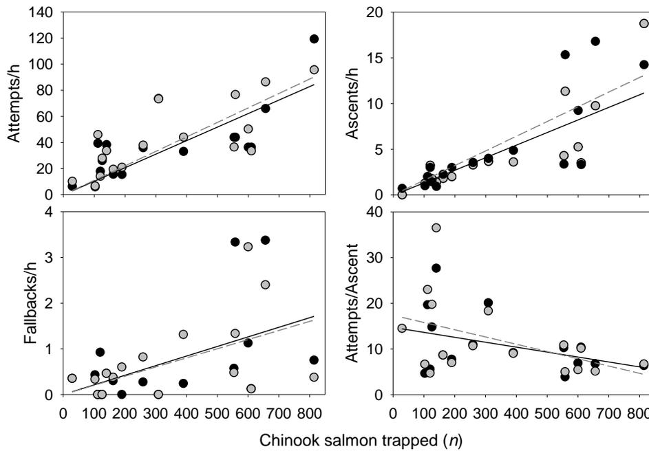
Figure 24. Relationships between the number of Chinook salmon processed at the Foster AFF and the behavior metrics calculated from optical video data collected at the pre-sort pool weir in 2017. Black and gray circles are estimates where the processing date was the final day or first day in each block, respectively. Lines are linear regressions forced through the origin for the hourly metrics.
