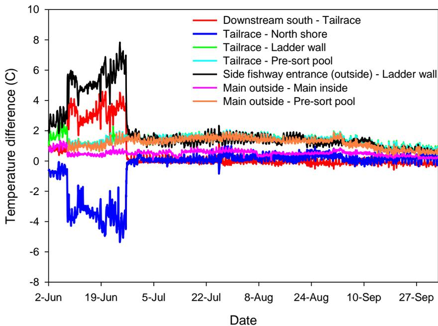
Figure 8. Pairwise differences in mean hourly water temperatures calculated from data collected at Foster AFF fishway and tailrace sites between 2 June and 3 October 2017. Site numbers as referenced in Figure A: Downstream south (12), Tailrace (9), North shore (1), Ladder wall (4), Pre-sort pool (10), Side fishway entrance outside (3a), Main outside (5c) and Main inside (5b).
