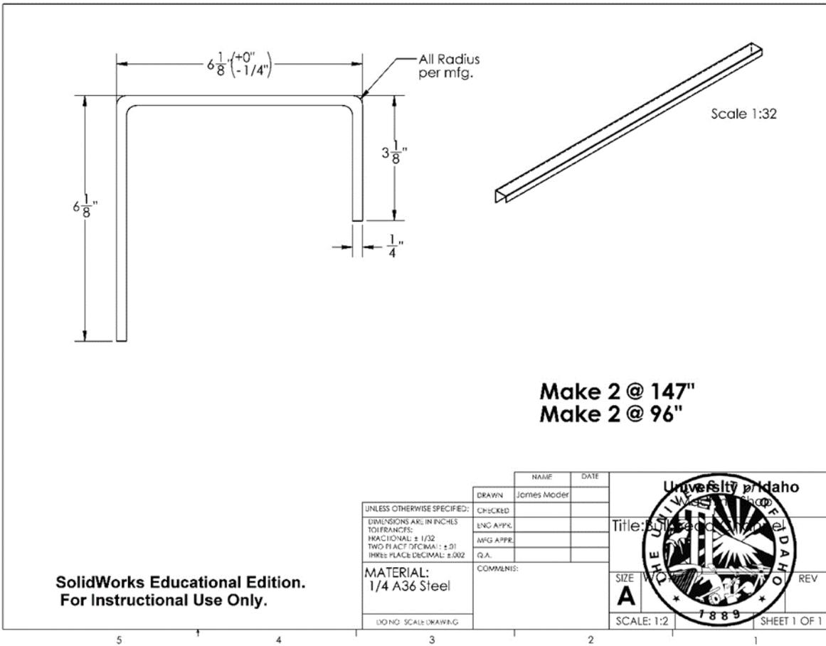
Figure A14. Bulkhead channel.
