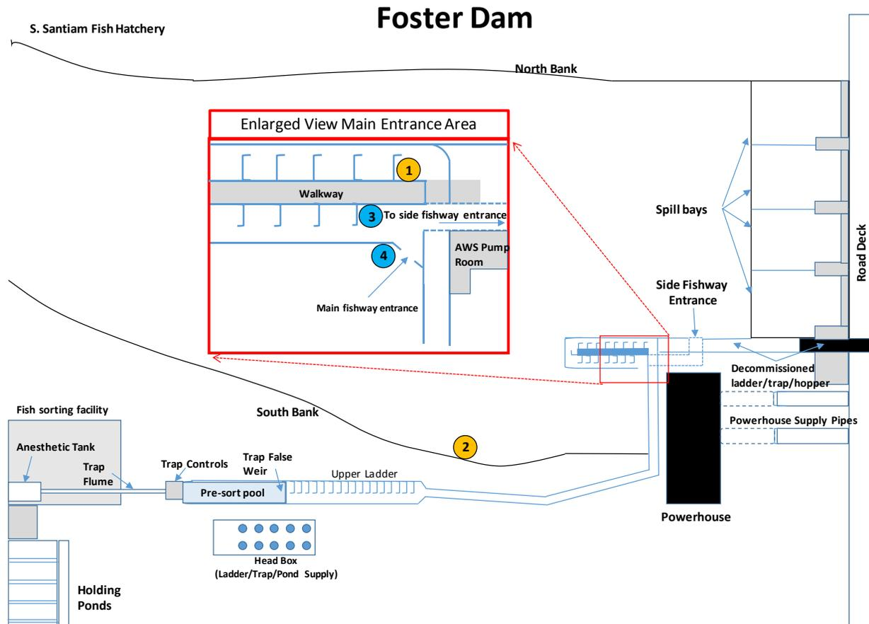
Figure 9. Map of the Foster Dam tailrace study area with location of hydrolabs (orange numbered circles) and water level loggers blue numbered circles in 2017. Hydrolabs: 1) ladder turn pool and 2) tailrace near south shore. Water level loggers: 3) inside the main entrance and 4) outside the main entrance.
