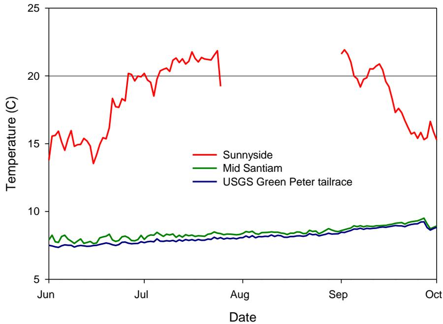
Figure 3. Daily mean water temperatures in 2017 in the Middle Santiam River. The loggers represent a progression upstream starting near the mouth at Sunnyside (rkm 426.8), to the Middle Santiam (rkm 430.0), and at the USGS site just downstream of Green Peter Dam (432.8 rkm). Solid line at 20 °C represents a threshold temperature considered to be physiologically stressful for adult salmonids.
