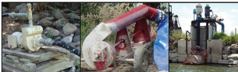
Figure 2. Examples of domestic, centrifugal, and turbine pumps.
