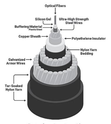
Parts of a submarine cable
