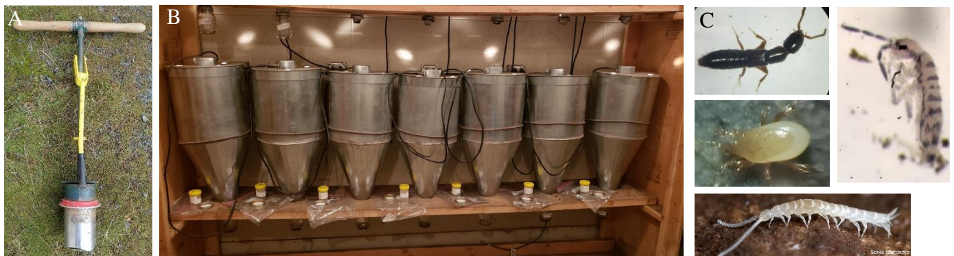
A) Soil corer used to sample soil arthropods; B) Berlese funnel system used to extract arthropods from soils; C) Example soil arthropods collected from the Soil Stewards farm
