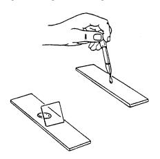
3. Holding a coverslip at a 45<sup>o</sup> angle, slowly lower it into the drop of water containing the letter. Preparing a slide in this manner is known as a *wet mount*. If properly done, there should be no air bubbles trapped under the coverslip. If this is not the case, start over again.
