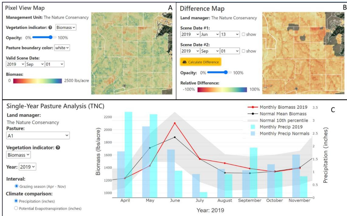
Figure 4. Select examples of RangeSAT ([rangesat.org](https://rangesat.org)) tools, which can inform use-based monitoring and adaptive management.
