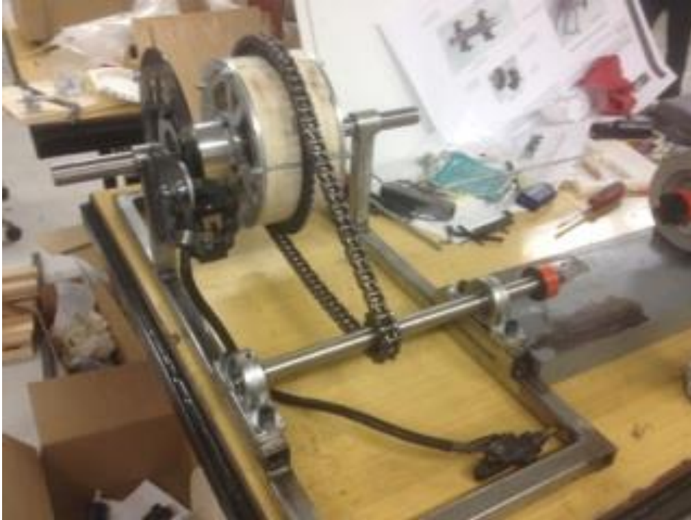
Figure 3-24: Final Assembly with wood mock up of the motor
