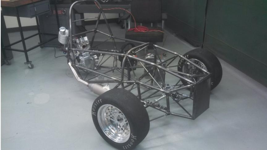
Completed chassis with completed front suspension, steering, and engine installed. Through the design and manufacturing process our team discovered which team members possessed certain gifts and skills. Moving forward utilizing each team member's specialties will help propel our project forward.
