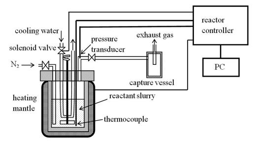
Reactor Schematic Diagram
