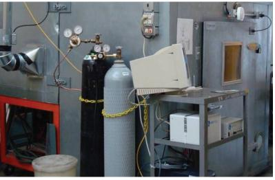
ments were carried out in a batch reactor system with precise temperature control. The content of microalgal methyl esters, the targeted product in the mixture after reaction, was analyzed by a gas chromatography-mass spectrometry (GC-MS). The product yield and the product selectivity were used as the indicators for process efficiency.
