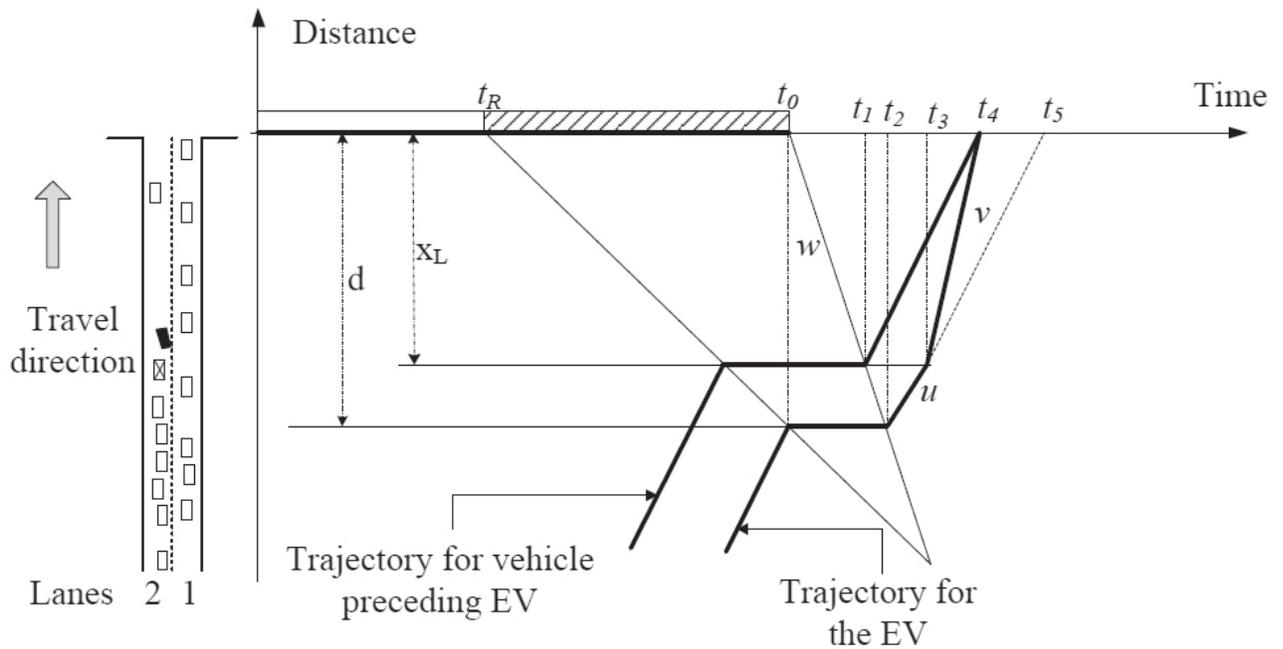
Shock wave profile of a single queue at a traffic light and the trajectories of the EV and preceding vehicle.
