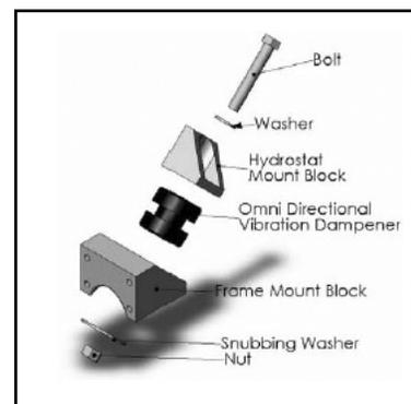
*Figure 5 Design of the hydraulic mount system.*
