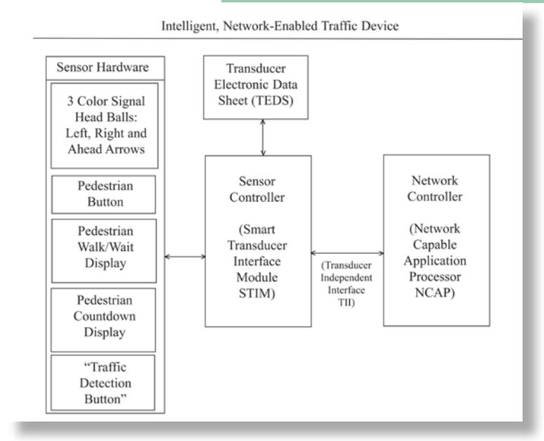
Figure 2. Design for an intelligent traffic network.
