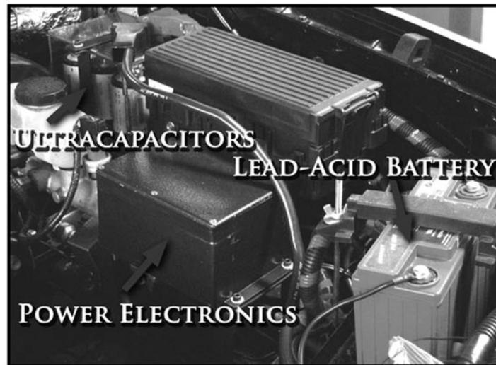
Figure 4 The system installation in a Ford Explorer consists of a bank of six capacitors weighing 0.42 lbs each, a DC/DC converter and controller and a small battery.
