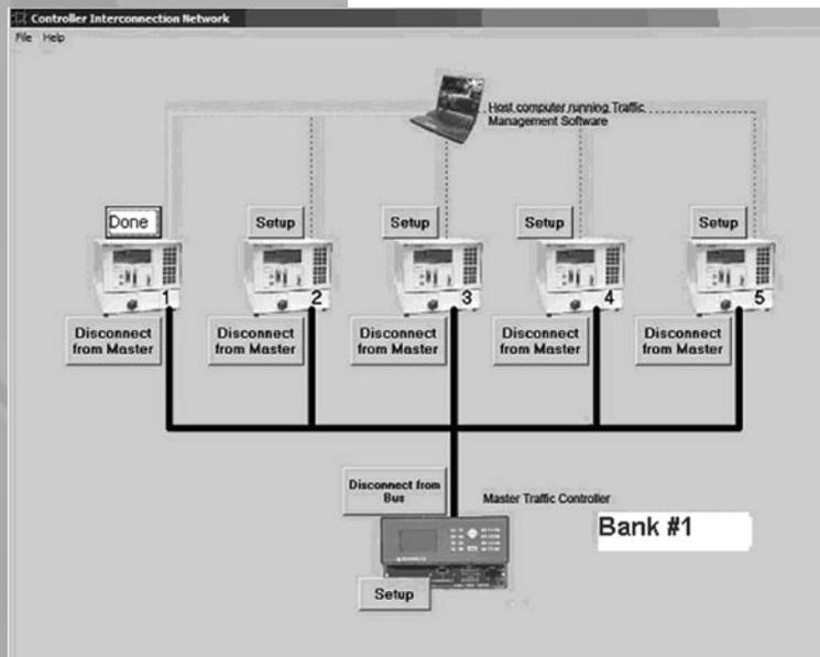
An embedded-controller approach was used for the hardware design because this approach enables easy modification. A GUI displays the status of the network and allows the user to make changes in network configuration.
