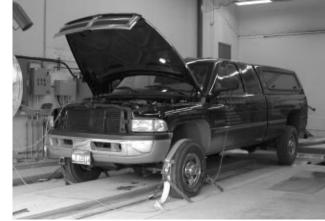
Biodiesel van undergoing testing on chassis dynomometer.
