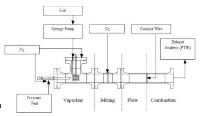
Schematic of the plug-flow reactor
