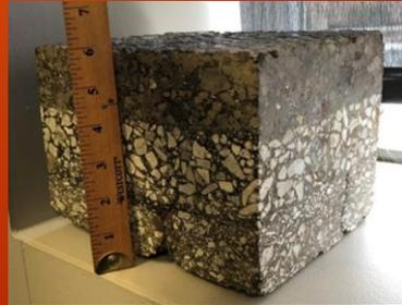
Steel Slag SMA Surface Course and Dolomitic SMA Intermediate Course
