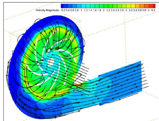
ANSYS Fluent Flow Simulation with Customized Pump Design
