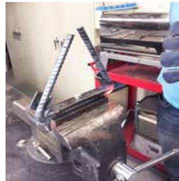
The triangle design consists of a 5-piece handle (left). Rebar was heated to bend the triangles into shape (above).
