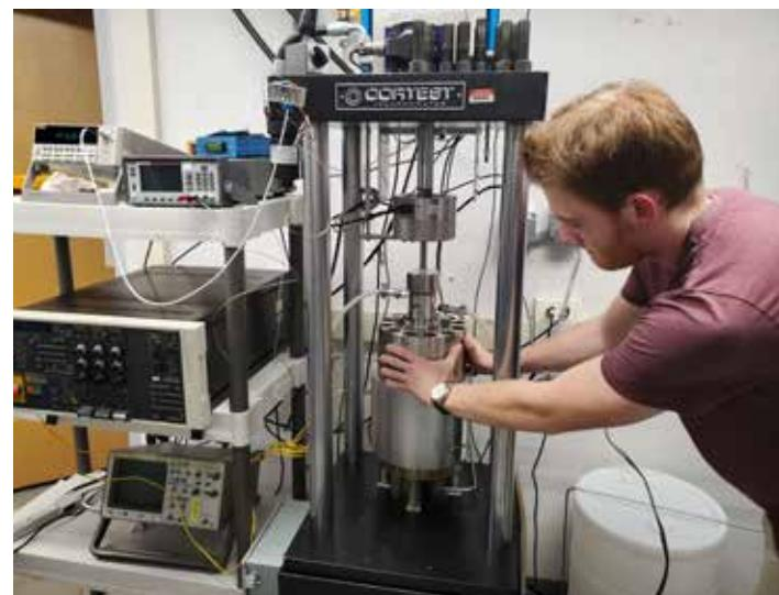
*Graduate student Colin Burkhalter demonstrates the apparatus designed to perform fatigue and corrosion tests at high temperature and pressure using a high purification water circulation loop.*
