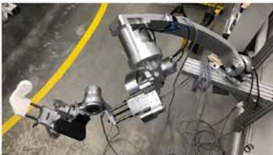
calculation, and motor commands are performed at a sufficiently high rate ( $\sim 1000$  Hz), the exoskeleton can effectively be used as an assessment instrument to measure user mobility, or provide assistive support forces.
