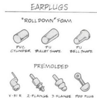
**Pre-molded earplugs** do not need to be rolled to conform to a worker's ear canal but the right sized earplugs must be used. They are relatively inexpensive, reusable, can be washed, require less handling, and come in a variety of sizes.
