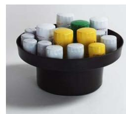
Terne-plated used oil filters do not qualify for the exclusion because the terne plating contains a tin/lead alloy. Terne may be used on filters found in heavy trucks or equipment. Collect these as a hazardous waste.
