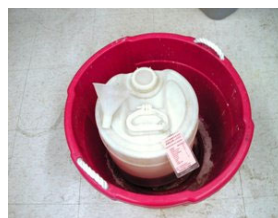
Plastic bucket for large items like carboys, especially if stored on the floor.
